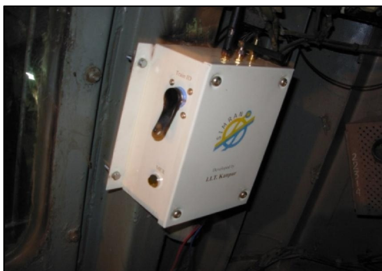
Figure 1: Box containing GPS equipment installed in trains Source: PPT from RDSO and IIT Kanpur
